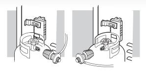
Loosen the cylinder lock wing nut. Swing the cylinder lock down. Tighten the wing nut.
